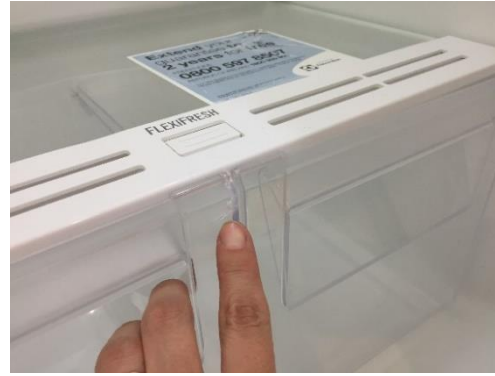
Small crack on the salad compartment
